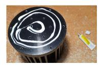
The heatsink has been tapped with M3 threads.
