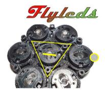
Important: Looking at the rear of the assembled lens frame, observe that the lens cups all have two small locating pins that will mate with the holes on either side of the LEDs, as called out by the horizontal line.
