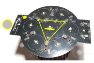
We have placed a small silver pen mark on the lens frame, as called out by the in the picture at left. This needs to be located closest to the Flyleds logo on the PCB.
