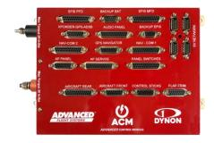
Advanced Flight Systems/Dynon supplies their Advanced Control Module or ACM as a component of their aircraft instrument panel wiring range. Along with many other features, the ACM provides power ports to drive:
