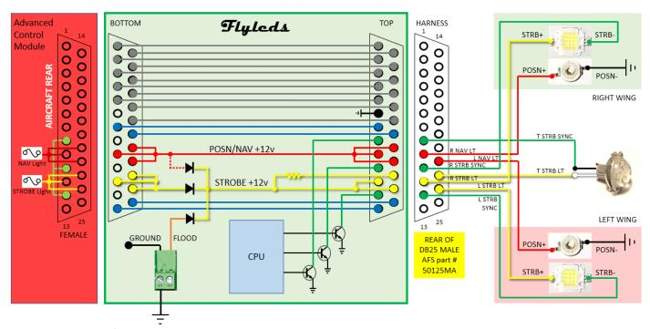
When the **Position/Nav light** switch is turned on, the ACM sends +12 volt power to the wingtip position lights via the red wires. The Flyleds CPU also energises the tail light at 10% power.
