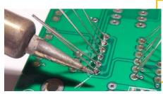
If the solder acts like it is 'allergic' to either the board or the resistor leg and does not want to flow smoothly around the component leg and the PCB pad, it is telling you that one part is not hot enough.
