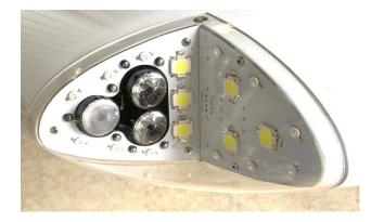
Finally, we have supplied you with two 20° beam diffuser disks. They fit into the 'north and south' key slots of the lenses. If you have the single spotlight boards wired and aimed as taxi lights you should find the resulting light spread more useful.
