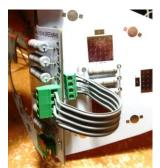
Ribbon wire has been supplied to interconnect the two wing boards. Trim away 1" of the webbing between each of the wires so you can strip the individual wires.
