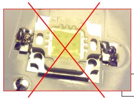
As the solder melts and flows, **if it acts like it is allergic to the PCB** or the LED leg then that part is not hot enough. Reposition the tip of your iron or give it a little more time (ie heat) and the solder should happily flow across both parts. (Who knew solder had a personality!)
