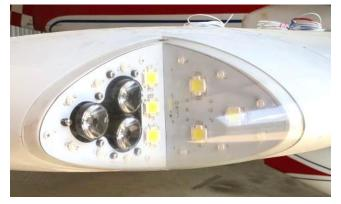
For a neater finish, the outward facing boards could be attached to the wingtip using thin double sided tape, such as carpet repair tape, or automotive tape as used to hold bump strips to car doors, for example. The prototype wing boards were installed in the wingtips a year before our RV-10's first flight, and then had to be pried off after 50+ hours of flying time when we replaced the boards with the production version. Three hundred flying hours later, the boards are not going anywhere!
