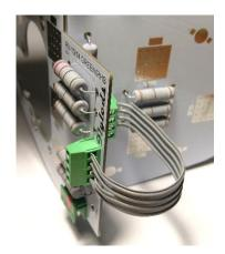
If you've just realised you've put the terminal blocks in facing the wrong way, **don't panic!**It all still works well with individual lengths of 20AWG wire rather than the supplied ribbon cable.
