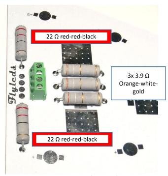
For the Green/RHS boards, the PCBs would sit on opposite places to that shown above, ie the forward facing spotlight board would be sitting on the right of this picture. Fit the  $12\Omega$  resistors (brown-
