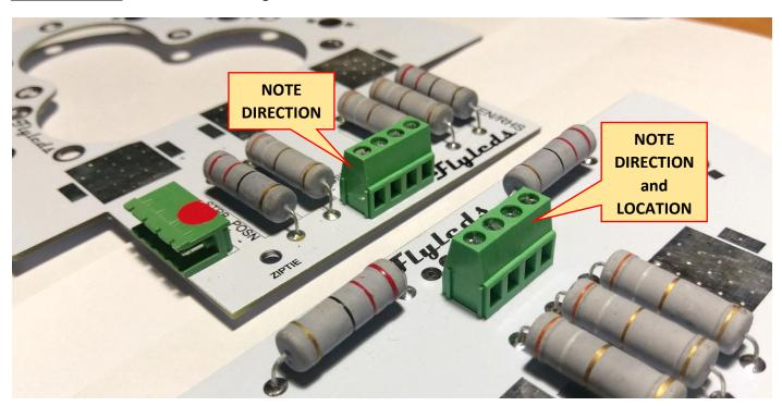
Note the position of the terminal block on the outward facing board. It goes in the holes closest to the resistors. This location allows room for the terminal block when it's inside the wing, as the two boards meet at an angle of about 70°.
