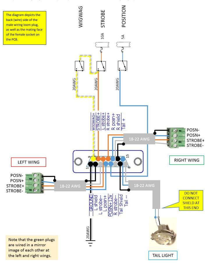
If you are replacing a conventional xenon strobe system this diagram shows how you can reuse the existing shielded wires, as well as the standard unshielded Position/Nav light wires as represented by the orange lines below.
