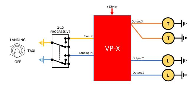
Using their configuration software set the VP-X to automatically wigwag the landing lights (output Y and Z) above a set airspeed. No warm-up time needed.
