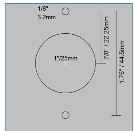
Drill the mounting screw holes and a 1 inch clearance hole in the appropriate rear-most position on your plane. The saddle clamp may then be bonded into position behind the fibreglass using a suitable adhesive. Due to the inconsistencies of the fibreglassing work on the inside of the fairing, some customers have cut the clamp into two smaller pieces and bonded each piece in the appropriate place.
