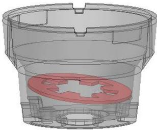
Place a lens locator ring inside the lens holder, shown at left in red.
