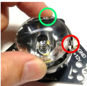
\* Rotate the PCB assembly/lens holder so that the locking hooks on the black lens holders are at **east** and **west** positions.
