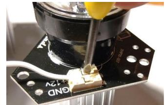
**Note:** The power connectors are suited for a **maximum of 18 AWG wire**. If you have 16 or 14AWG wire already in your plane, either splice a short length of 18 or 20 AWG to the end of your wire run, or simply peel out and trim off a few strands of wire to reduce its diameter. The connectors are not designed for repeated use, so an additional inline plug/socket of your choice may be used here as well.
