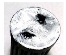
**Wait ten minutes or so.** If any excess glue has oozed through the holes close to the LED, carefully scrape it away with a small screwdriver. Use less glue next time!
