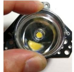
below. This indicates that the LED and lens are in alignment.
