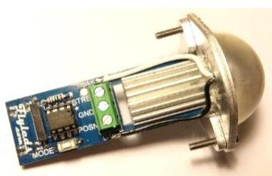
If you have purchased our Stand-Alone tail light with the integrated circuit board, wire it directly to your Strobe and Position light switches on the panel, and ground it locally at the tail. Do not connect it to the Controller Board.
