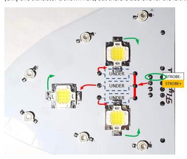
At the wings, strobe 12 volt power comes in on the STRB+ terminal on the green terminal block.
