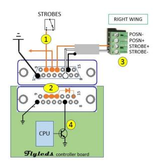
(4): The CPU on the controller board turns on the small switching MOSFET transistors in sequence. This connects the STROBEwire to ground which turns the LEDs on.
