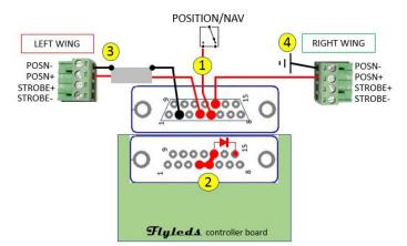
On the wing boards the position LEDs are wired in series in a group of three LEDs, one group along the top of the board and one along the bottom. If one LED is installed backwards all three LEDs in that group won't light up.
