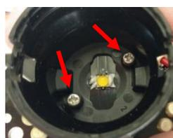
Fit two M2.5 machine screws into the holes in the lens holder and attach the heatsink to the board.
