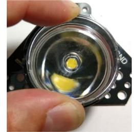
Using even pressure from two fingers from your other hand on the east and west sides of the lens, push the lens in gently until it clicks into place under the tabs at the left and right sides of the holder.
