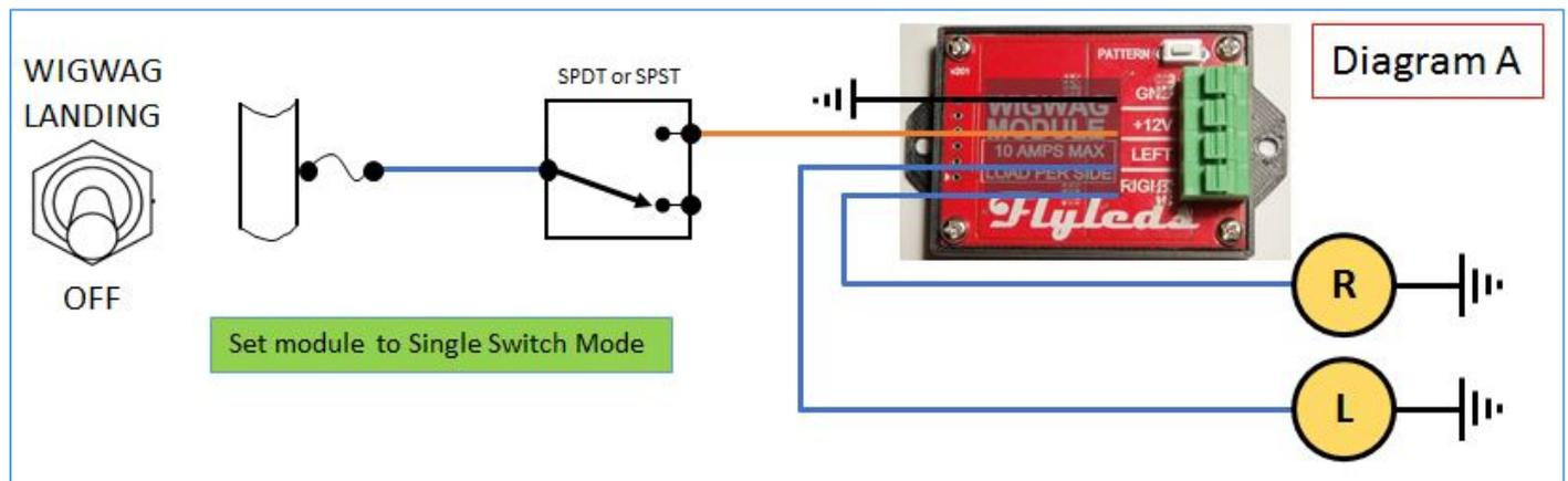
**To enable this mode** of operation, press and hold the PATTERN button and then apply power. Release the PATTERN button. Both landing lights will flash briefly and then come on continuously as you would expect.
