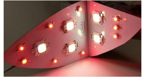
The forward facing board only has two strobe LEDs, and room for only three red or green position LEDs. This is less than our other kits, but still exceeds minimum strobe and position lighting requirements in all directions. And you'll still need eye protection when they are on!
