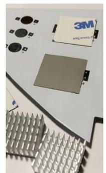
Don’t forget to *remove any red and green dots* once you’ve mounted the boards to your wings. And if you have a nice shiny red/lime green/purple plane, you can always mask up each LED with low-tack tape and spray paint the circuit board to match. Be careful when removing the tape from the position LEDs as it is possible to damage the dome of the LED.
