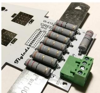
We use a steel ruler to keep the resistors a nice consistent 1mm or so height above the board to allow for air flow.
