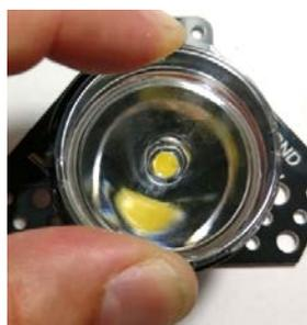
As you lower the lens straight down into the holder you will observe the centre of the lens begin to change colour to yellow from the LED below. This indicates that the LED and lens are in alignment.
