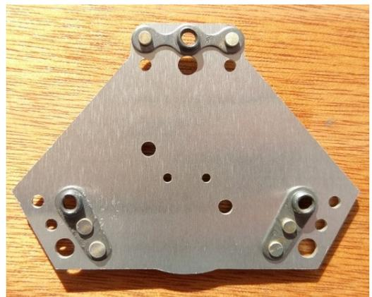
Next fit the lens holder onto the light board. Note that the holders have two tabs in their base. These fit into the small holes above and below the LED, and will locate the holder and lens in the optimum focal point for the LED.
