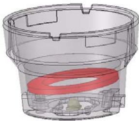
Place an Anti-Decapitator Ring™ inside the lens holder, shown here in red. It may be slightly oversized and not sit flat. This is OK! Developed by Flyleds in response to some customers damaging the LEDs (and we admit we've also done it ourselves), the Anti-Decapitator ring is designed to flex and it will guide the lens into the correct position in the following steps.
