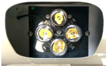
We attached the independent LED after the main board was fitted to the Duckworks mounting plate, which meant we didn't have to make any modifications to the existing metalwork or the Combo light itself. If you have the option to do this, removing the wingtip is 30 minutes well spent and makes life much easier!
