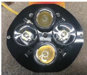
Held at the right angle to the light, you will observe that the circuit board traces form a 100mm diameter circle around the lights, while the rest of the perimeter of the board is vacant. Feel free to trim, drill or otherwise modify the outside area of the board if you feel the need!
