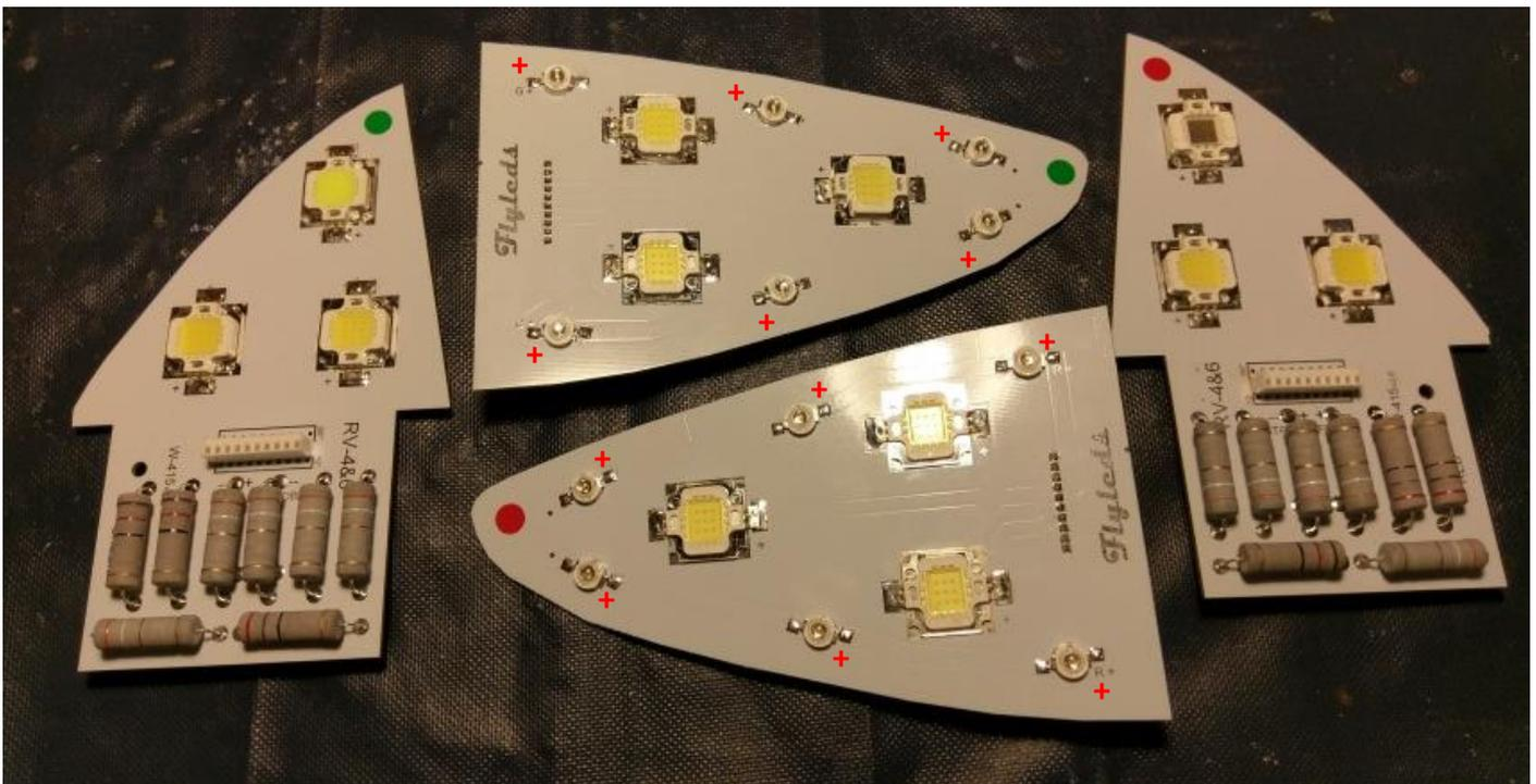
If you choose to fix the boards to your wing with screws, avoid drilling through any track lines by choosing a more 'open' area of copper. We used automotive double-sided trim tape instead for our RV-10 with great success. Even after a few hundred flight hours, they aren't going anywhere.
