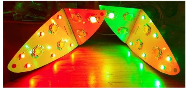
The forward facing board only has two strobe LEDs, with the third LED being either a red or green 10W rated position LED. This is one less strobe LED than our other kits, but you'll still need eye protection when they are on!
